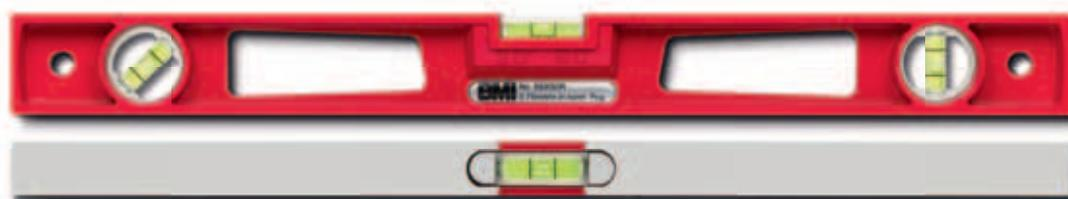
Aluminum die-cast level, milled on all sides, red powder-coated. Highly torsion resistant. Handles for easier handling. 45° vial. Accuracy in normal position 0.75 mm/m.
