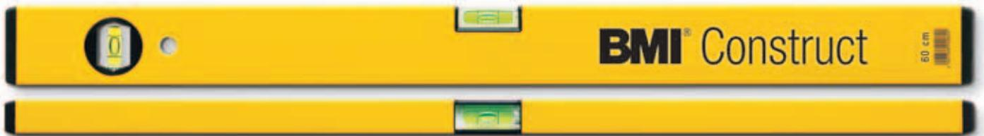
Sturdy level with crack resistant plastic vials. Robust, smooth aluminum profile, yellow powder coating. Measuring accuracy in normal position 1 mm/m.
